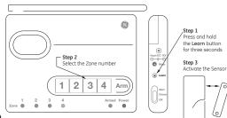
Step 2 - Press the Zone button (1, 2, 3 or 4) for the Zone you want to assign to the Sensor. The LED indicator for that Zone will begin to flash.
